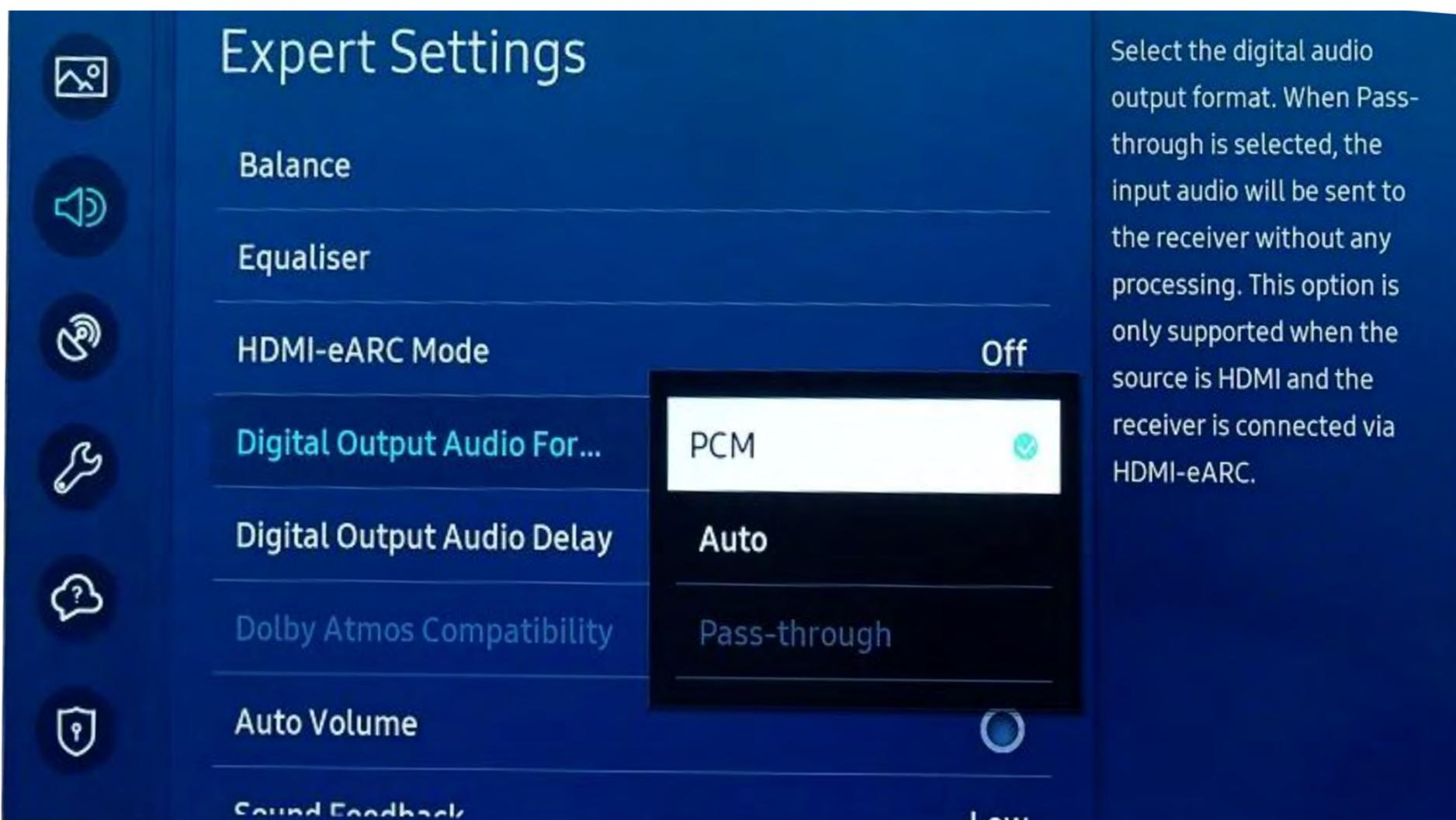
Select the digital audio output format. When Pass-through is selected, the input audio will be sent to the receiver without any processing. This option is only supported when the source is HDMI and the receiver is connected via HDMI-eARC.
